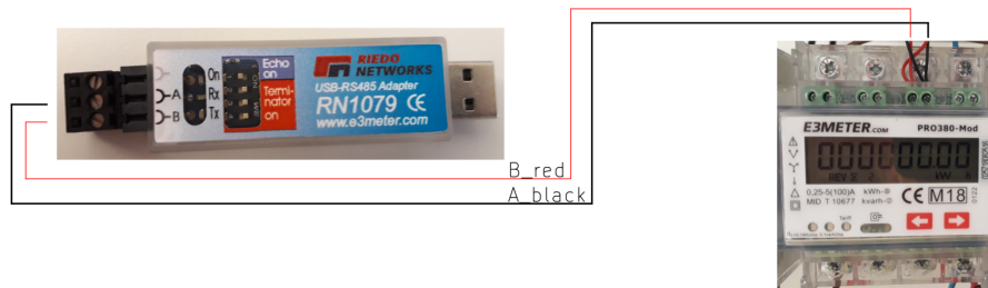
Fig. 5: PRO meter connection per USB adapter on CTR
